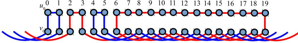
Figure 9. Two spanning cycles for  $GP(4r, 4)$  for  $r = 5$ .
