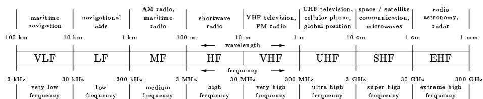
Figure 1: The radio spectrum applicable for wireless communication
